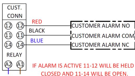
Figure 7: FPS-900 Alarm Contact Diagram
