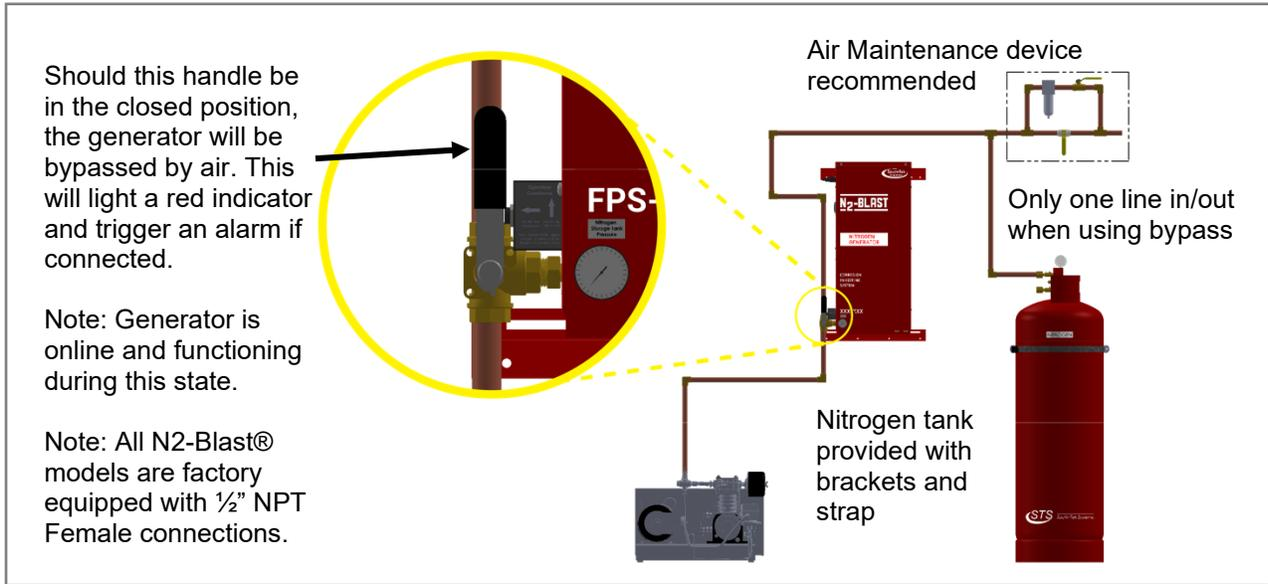
**Figure 3: Nitrogen Generator Wall Mount Installation Setup**
