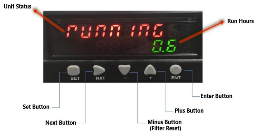
**Figure 6: Controller Display**
