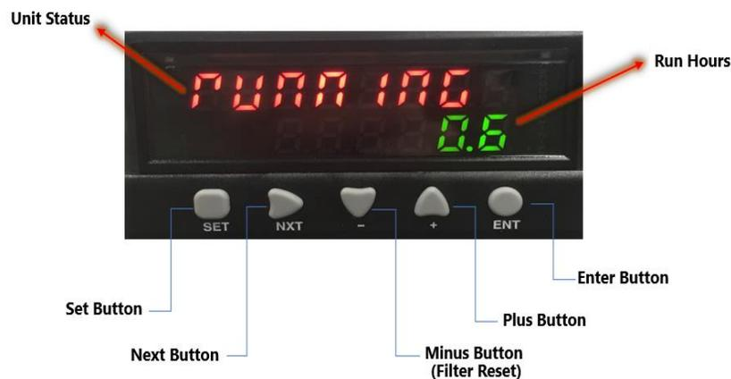
**Figure 6: Controller Display**
