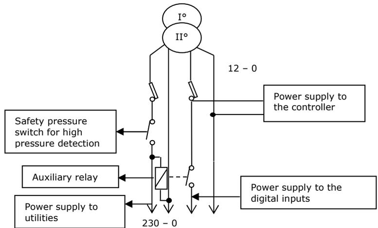
**Note:** Although Ozen Air Technology does not use a safety pressure switch in conjunction with the Maestro 22, it is important to note that the **"SAFETY PRESSURE SWITCH"** alarm (A21) is still active and will be issued if all the digital inputs are open.
