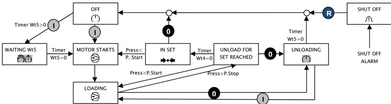
The symbols in the above squares indicate the compressor status showed on the main visualization of the LCD. The back is grey while the symbol is blinking.
