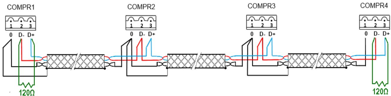
**IMPORTANT! Incorrect wiring can damage both the controller and any other devices connected on the serial net.**
