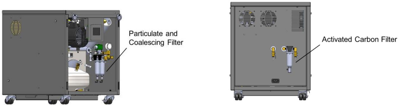
Figure 23: LABTEK™ N2-35 Series Filtration Units
