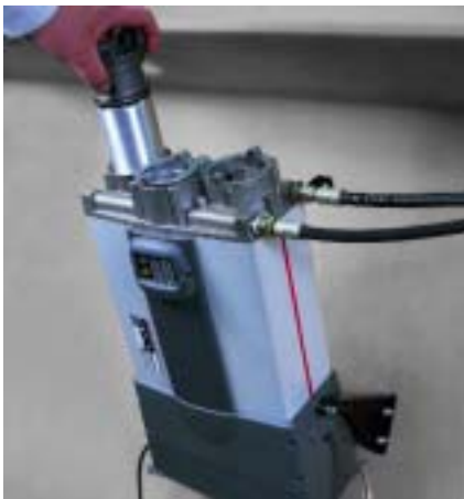
Tilt mounting kit facilitates easy cartridge replacement in restricted access applications
