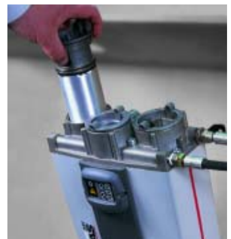
Easy desiccant cartridge replacement
