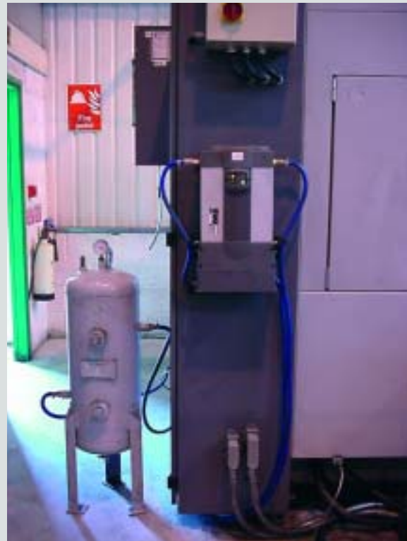
PNEUDRI MiDAS installed to supply control air for a CNC machining center
