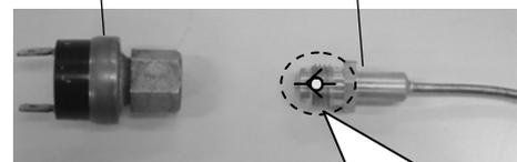
There is a check valve built into this fitting. When it is screwed into the pressure switch, this valve opens. When removing or attaching, if it is not done quickly, refrigerant gas may leak out.
