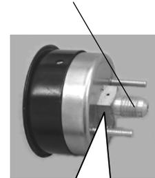
Use a spanner to hold the square part of the base of the refrigerant connection screw and remove the piping flare nut
