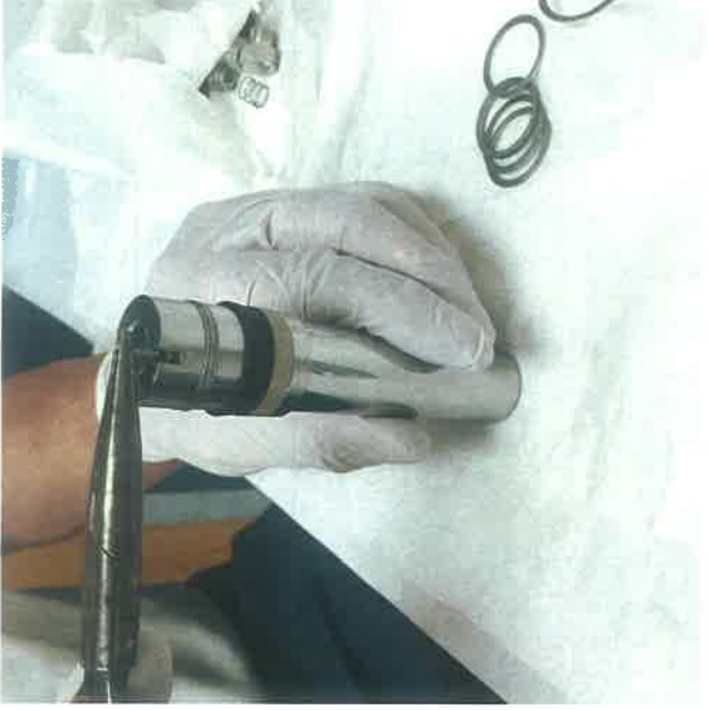
FIGURE 1-9. COTTER PIN BENT UPWARD 90 DEGREES
