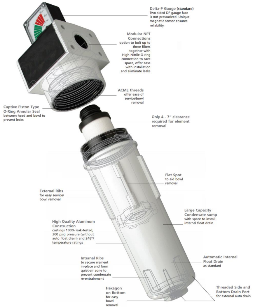
Figure 37: Filter Element Change for some CS Series and S Series
