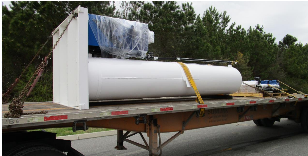
Figure 2: Generator Strapped to Flatbed
