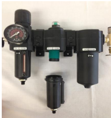
Figure 4: Coalescing Filter Element Replacement
