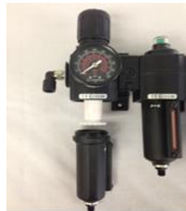
Figure 3: Particulate Element Replacement
