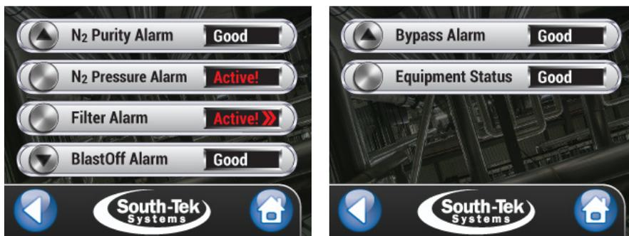
Figure 20: Alarm Menu Screens (O<sub>2</sub> Purity with presence of O<sub>2</sub> Sensor)
