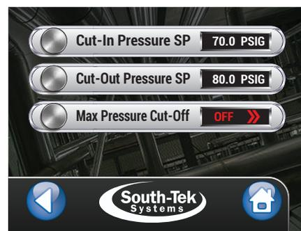
Figure 23: N<sub>2</sub> Pressure Settings Screen
