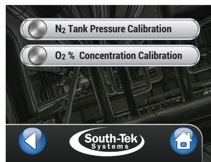
Figure 24: Sensor Calibration Options Screen (O<sub>2</sub> will show in the presence of O<sub>2</sub> Sensor)
