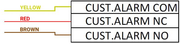
The yellow wire acts as the common which will supply power to the NO or NC depending on alarm status. If an alarm is triggered, including BlastOff<sup>TM</sup>, filter replacement, and compressor replacement, the COM and NO will be connected, and the COM and NC will be disconnected. The NC connection (red) also acts as a power loss indicator, it will signal if the generator is unplugged or accidentally turned off.
