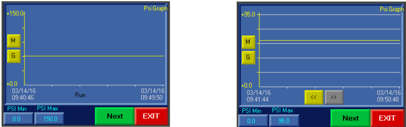
Figure 3: Left - Graph Screen, Right, Graph Screen with History Scroll and Grid Lines
