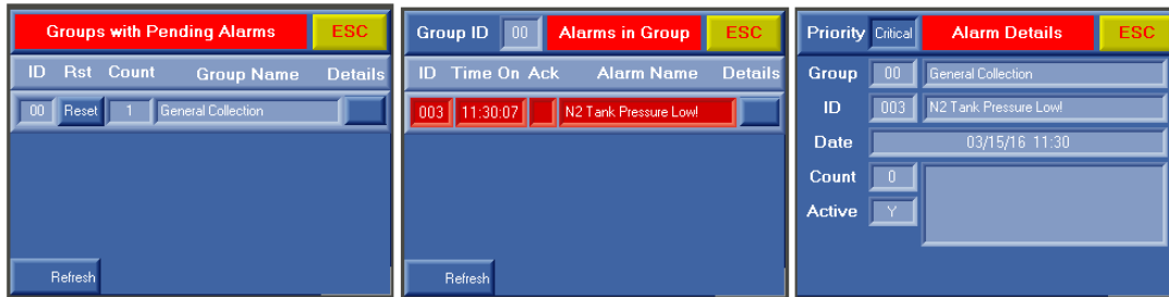
Figure 9: Alarm Detail Screens (Button below "Details" Column Brings up the Next Screen)
