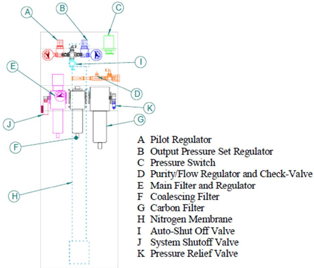
**All Settings are Factory Set and should not be changed in the field without proper diagnostic equipment. Any changes to the regulators will affect the performance and purity of the system's output and could damage the system.**
