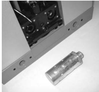
5. Silencer can be thoroughly cleaned in warm soapy water. Do not use sharp instruments or tools.
