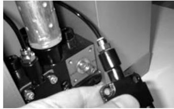
5. Disconnect tubing from fitting on bonnet.
