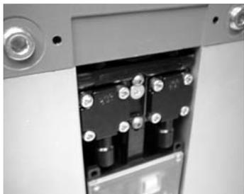
1. Remove front panel of dryer as described in 11.5 and locate purge plug in upper valve block.
