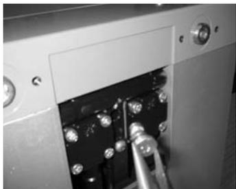
3. Remove purge plug from port in upper valve block downwards.
