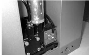
6. Locate diaphragm assembly to be changed.
