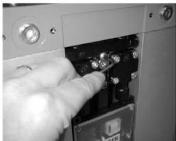
2. Remove purge plug fixing screw from upper valve block.
