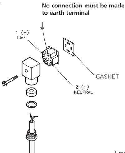
3. The dryer is double insulated therefore no earth is required.
