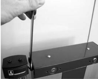
1. Inlet filter is fitted to dryer in vertical orientation. Loosen fitting.
