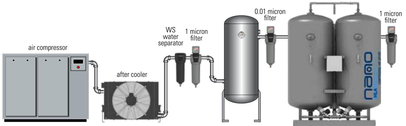
Installation is suggested when the compressed air treated from the dryer is only a part of the total flow rate of the compressor; or when the compressor operates at reduced load and the total consumption equals the compressor flow rate.
