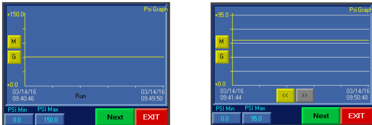
Figure 7: Left - Graph Screen, Right, Graph Screen with History Scroll and Grid Lines
