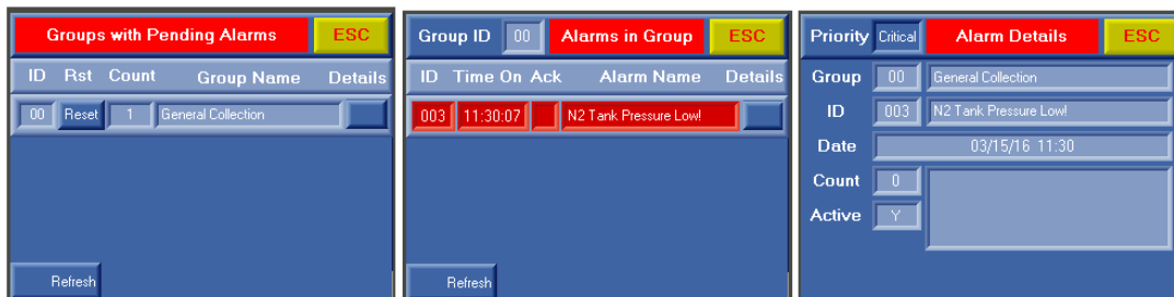
Figure 12: Alarm Detail Screens (Button below "Details" Column Brings up the Next Screen)
